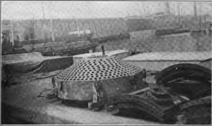
FIG. 135.—Parts of a 10 ft. 6 in. diam. calandria vacuum pan. Calandria of cast brass, 10 ft. 0 in. diam., weighing 9000 lb., with tubes expanded-in.
